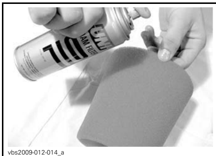
TYPICAL - OIL THE FOAM FILTER ELEMENT
