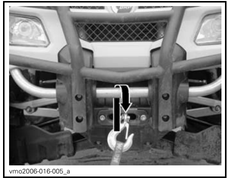
TYPICAL — FRONT TIE-DOWN POINT LOCATION
