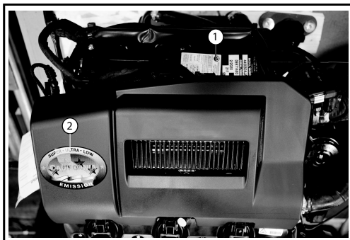
TYPICAL TOP OF ENGINE (BEAUTY COVER INSTALLED)
