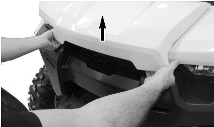
LIFTING FRONT SERVICE COVER EDGE.
