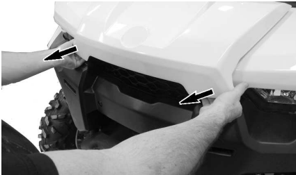
PULLING ON FRONT SERVICE COVER EDGE.
