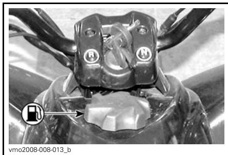
TYPICAL — FUEL TANK CAP
