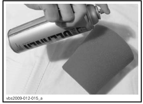
TYPICAL - SPRAY FOAM ELEMENT INSIDE AND OUT
