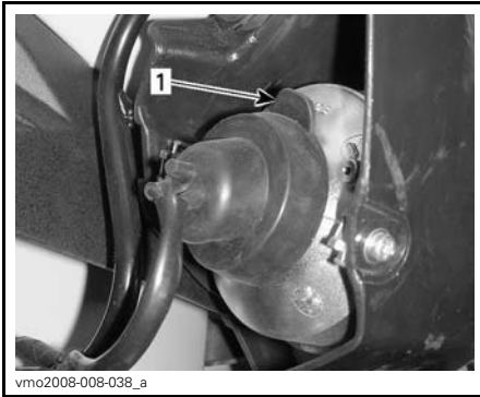
REMOVE RUBBER PROTECTOR 1. Rubber protector
