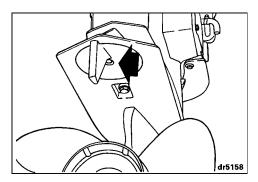
Tighten the trim tab screw to a torque of 35-40 ft. lbs. (47-54 N·m).
