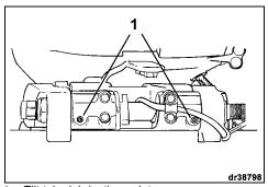
1. Tilt tube lubrication points
