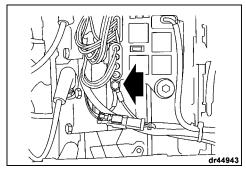
**IMPORTANT:** The accessory battery connection must only be used to charge a single 12-volt battery or two 12-volt batteries wired in parallel. The accessory connection must not be used to charge either battery in a 24-volt system.
