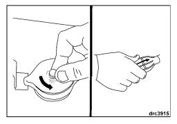
If equipped with an electric fuel primer pump, activate it for about 20 seconds.
