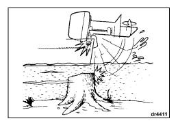
The engine's shock absorption system does not work while operating in reverse. If you back into an object, either in the water or while trailering, your boat and engine can be seriously damaged.
