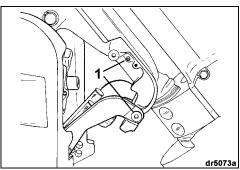
1. Trailering bracket lubrication points
