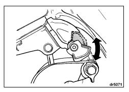
Disengage the tilt support lever:
