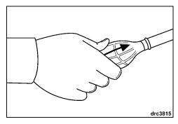
**IMPORTANT:** Fuel distribution hoses in the boat must deliver fuel at the rate of flow needed by the engine. Minimum inside diameter of fuel hoses must be 3/8 in. (9 mm).
