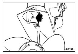
Tighten the trim tab screw to a torque of 47-54 N·m (35-40 ft. lbs.). Test the boat and, if needed, repeat the procedure until steering effort is as equal as possible.
