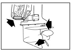
Galvanic corrosion destroys underwater metal parts and can occur in fresh or salt water; however, salt, brackish, and polluted waters will accelerate corrosion.
