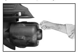
Remove the cotter pin and loosen the impeller nut. Remove the nut, spacer, impeller, and thrust bushing.
