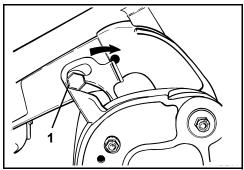
Tilt support bracket – unlock position
