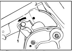
Tilt support bracket - lock position
