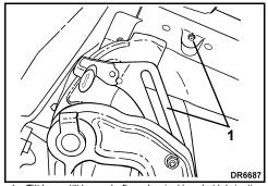
Tilt lever, tilt lever shaft, and swivel bracket lubrication points (annually)
