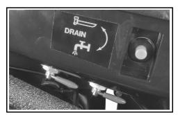
**IMPORTANT:** DO NOT run the outboard with the drain valves in the DRAIN position more than 3 minutes. Engine damage can result.
