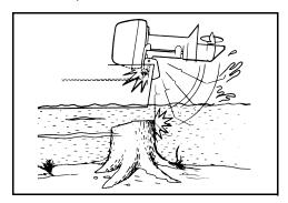
**NOTICE** The outboard's shock absorption system does not work while operating in reverse. If you back into an object, either in the water or while trailering, your boat and outboard can be seriously damaged.
