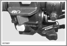
CHOKE LEVER IN THE OFF POSITION The full choke position is used for lower engine temperature.
