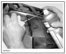
**NOTE:** Place a rag around the throttle cable adjuster to prevent the lubricant from splashing.
