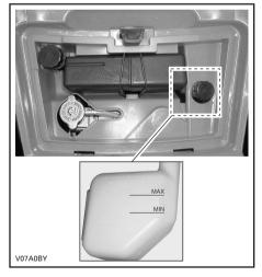
With vehicle on a level surface, liquid should be between MIN. and MAX. level marks of coolant reservoir.
